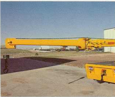
Self-storing boom extension provides 10 ft. of additional length.
