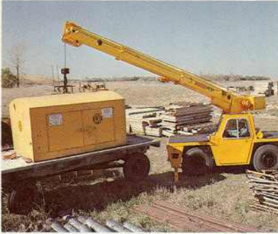
Maximum capacity 16,000 lbs. anywhere within 360° continuous rotation.
