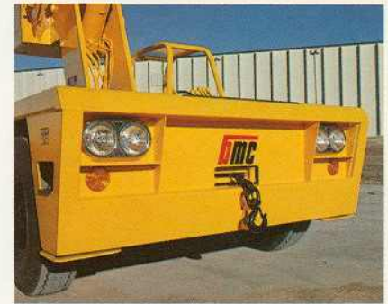
An optional auxiliary winch may be mounted behind the front bumper.
